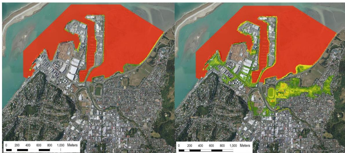
Figure 7-3: Areas of The Wood and CBD inundated by a MHWS-6 water level under a RCP8.5+SLR scenario by 2070 (left) and 2130 (right)
