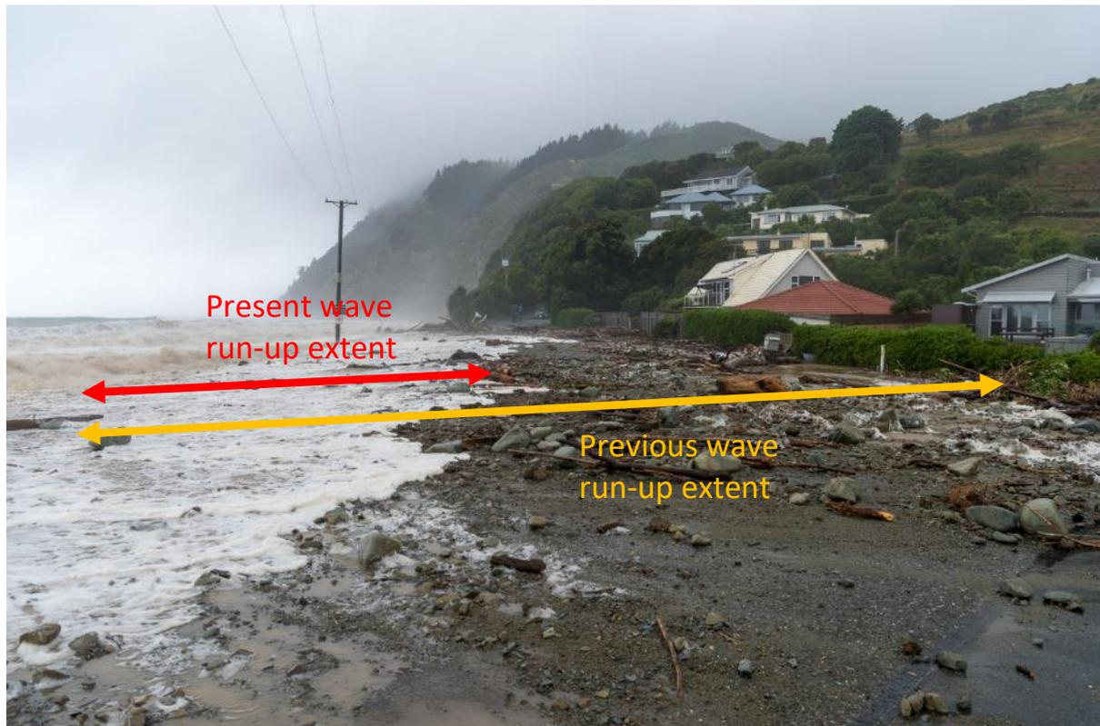
Figure 3-5: Photograph at Glenduan (taken 1 February 2018) showing extent of previous wave run-up
