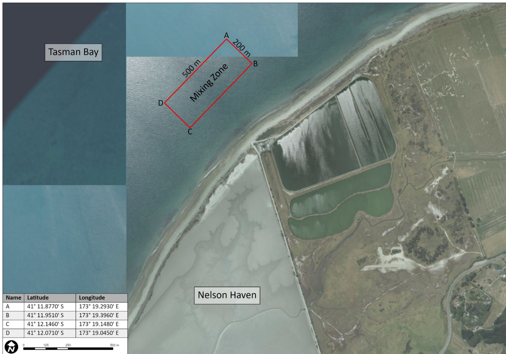
Figure 2. The extent of the mixing zone is defined as the area delineated by a rectangle measuring 500 metres by 200 metres centred on the outfall diffuser structure. The coordinates presented in Figure 2 relate to the mixing zone for the existing outfall diffuser structure. Condition 20 states that if any replacement outfall diffuser constructed, as provided for in Condition 24, results in the centre point of the new diffuser being in a different location to that of the existing outfall diffuser, then the mixing zone rectangle must move so that it centred on the middle of the new outfall diffuser, and this will change the coordinates presented in Figure 2.
