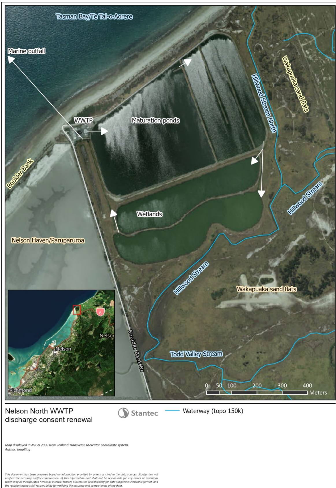
Figure 3-1: Overview of the NWWTP and surrounding environment. The overview includes labels for the main aspects of the WWTTP (white text) and indicative flow direction through the WWTTP (white arrows). A tabular representation is provided within Table 1
